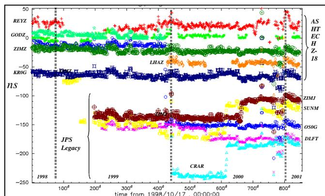
Fig. 9: GPS-GLONASS receiver bias for several stations.
